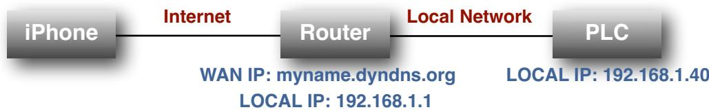
First determine the LOCAL IP address of the GPRS or ADSL router. PLCs need to know the router address as it is the gateway to the internet.
