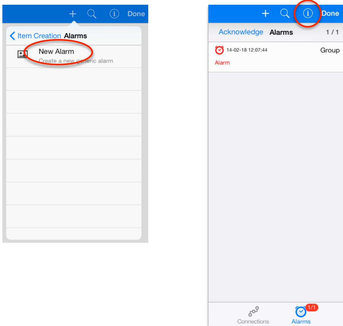
When an alarm condition is triggered, alarm information such as their *group* and *comment* properties are displayed in an ordered list on the Alarms Viewer. Alarms will remain on the list as long as they are active or otherwise if they have not been acknowledged. Their current state is shown by small icons next to the alarm text:
