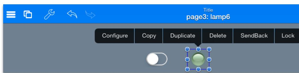
By entering the *switch.value* into the *value* property of the *lamp* we achieve the desired effect because when the *switch* changes a change event will propagate a change to the *value* property of the *lamp*
