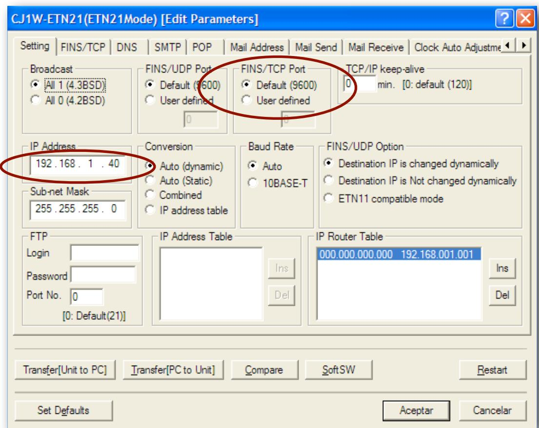
2. For **EIP/Native** protocol and Allen Bradley controllers use RS-Logix 5000 tool to set a fixed local IP for the PLC on the ethernet module properties panel.
